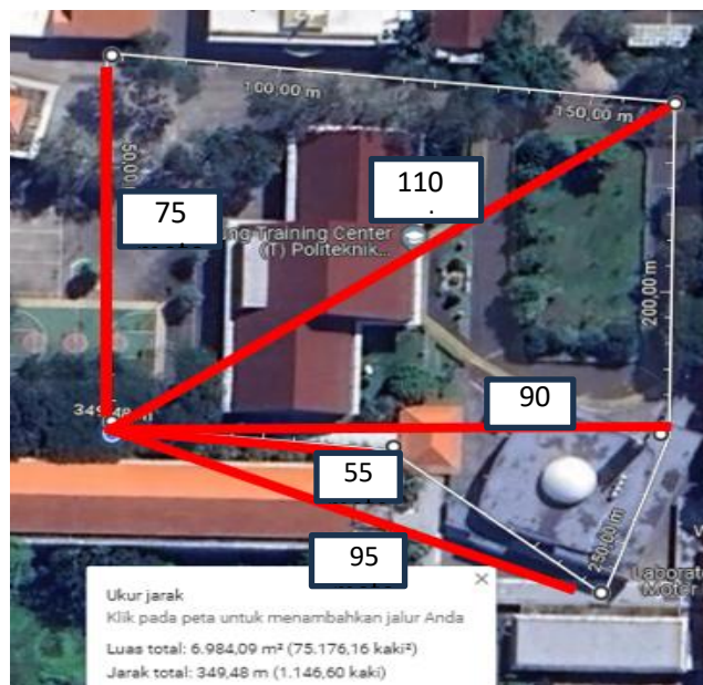
Gambar 4. Denah Pengujian Integrasi MQTT-LoRa
