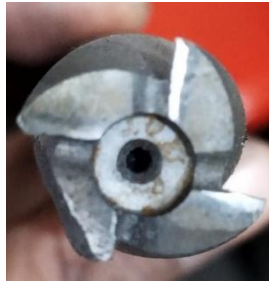
Gambar 7. End Mill Cutter Rusak
